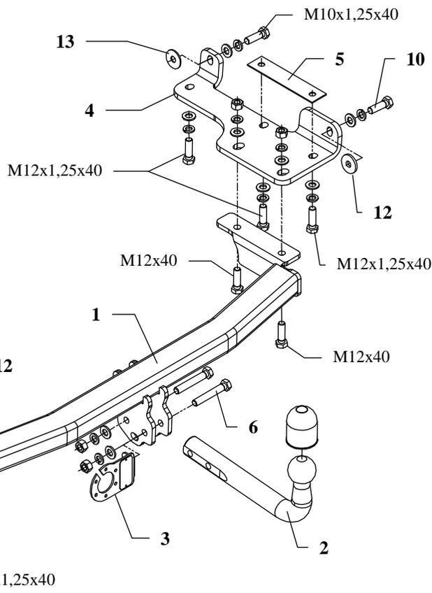
This towbar is designed to assembly in following cars: **NISSAN MURANO (Z50)**, produced since 11.2004 till 2008, catalogue no. **V62** and is prepared to tow trailers max total weight **1500kg** and max vertical load **100 kg**.
